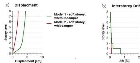
Figure 8. a) Diagram of floor movements of both models b) diagram of relative floor movements of both models
