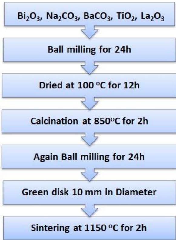
Figure 2.1 Flow chart of solid state route method for La-doped BNBT ceramics.
