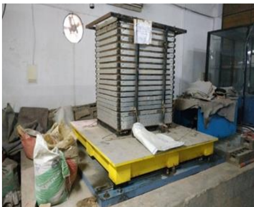
Figure 2: shaking table facility (Chakraborti, 2021)
