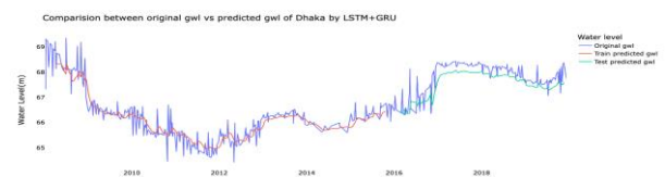
Figure 19: Comparison between original GWL vs predicted GWL with chart of Dhaka by LSTM+GRU
