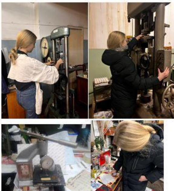
Fig. 2.2. Work near the tearing machine ID-1 (on the left), press machine L.Shopper Fig. 2.3. Working with PIM microhardness-tester and with Durometer (right).
