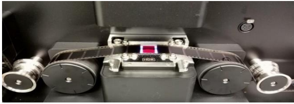
Figure 1 Scanning a 35mm motion picture film
