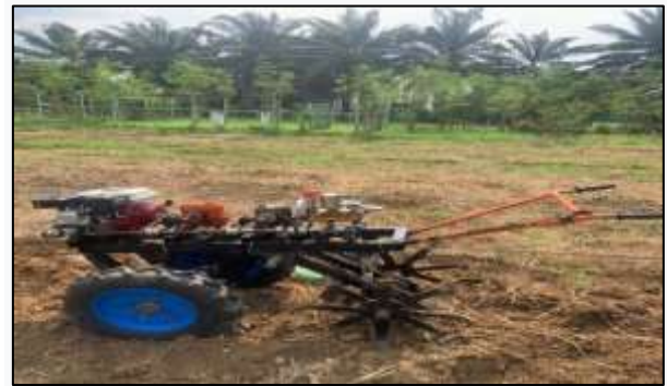
Figure 9 Mini Tractor Test Measuring Speed on Dry Land.
