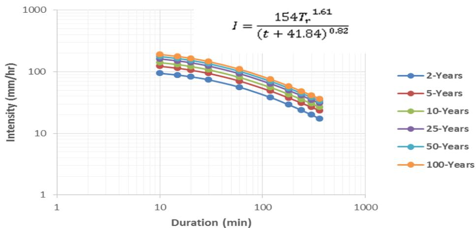
Figure 3.4: IDF curves by LPT III method at Owerri (South-East Nigeria)
