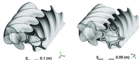
Figure 1. Grids for first stage (top) and second stage (bottom) of the compressor
